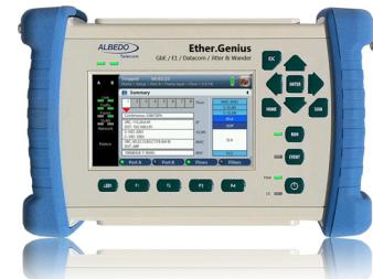
Once **mobile backhaul** has migrated to Ethernet/ IP / MPLS a bunch of synchronization alternatives are available including: a) **TDM** based signals such as E1/T1, b) satellite based **GPS** and c) packet based solutions such as **SyncE** and **PTP**. **Ether.Genius** is suitable for testing all this three environments and also those hybrid architectures on packet have not totally replaced legacy circuit switching.
